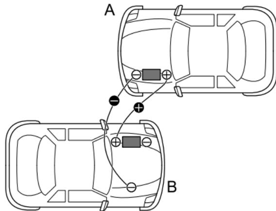
Ensure the START/STOP Switch is turned off and switch off ALL electrical equipment of BOTH vehicles, then follow the instructions below:
