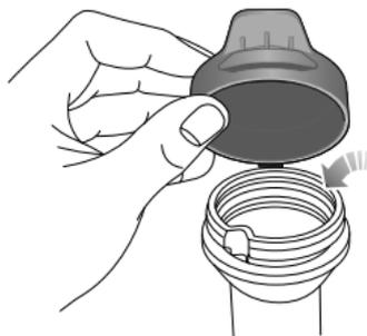
Check the washer fluid level every week. When the level of washer fluid is low, please top up the washer fluid as instructed.
