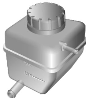
The cooling system should be checked weekly when the cooling system is cold and with the car resting on level ground. If the coolant level is below the "MIN" mark, open the coolant expansion tank cap and top up coolant. The coolant level should not be higher than the "MAX" mark.
