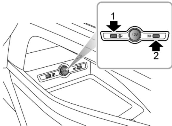
The 12V front console power socket is located in the storage box in front of the shift control knob. When the START/STOP Switch is in the ACC or ON/READY positions, it can be used as a power supply.
