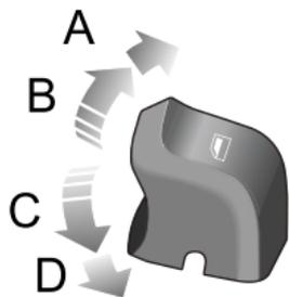
Press the window control switch (2 ~ 5) to the first position (C) to lower the window; Lift the switch to the first position (B) to raise. The window will stop moving as soon as the switch is released.
