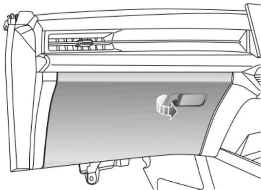
To open the glove box, pull the handle on the glove box cover (as indicated by the arrow).
