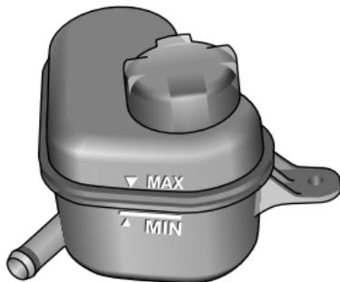
The cooling system should be checked weekly when the cooling system is cold and with the car resting on level ground. If the coolant level is below the "MIN" mark, open the coolant expansion tank cap and top up coolant. The coolant level should not be higher than the "MAX" mark.
