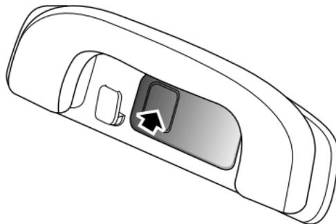
The rear interior lamps are located on the left and right sides of interior roof panel. Press the lamp lens as indicated in the diagram to switch on the rear interior lamps, press it again to switch off the lamps.
