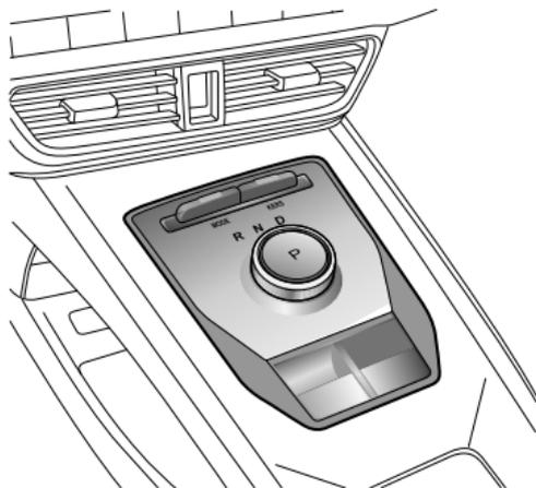
The shift control knob defaults to the intermediate steady state position, there are two unsteady positions clockwise and counterclockwise, the shift control knob will return to the intermediate steady state position once released.
