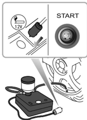
**Note:** To avoid battery discharge, it is recommended to keep the vehicle in P and READY mode.
