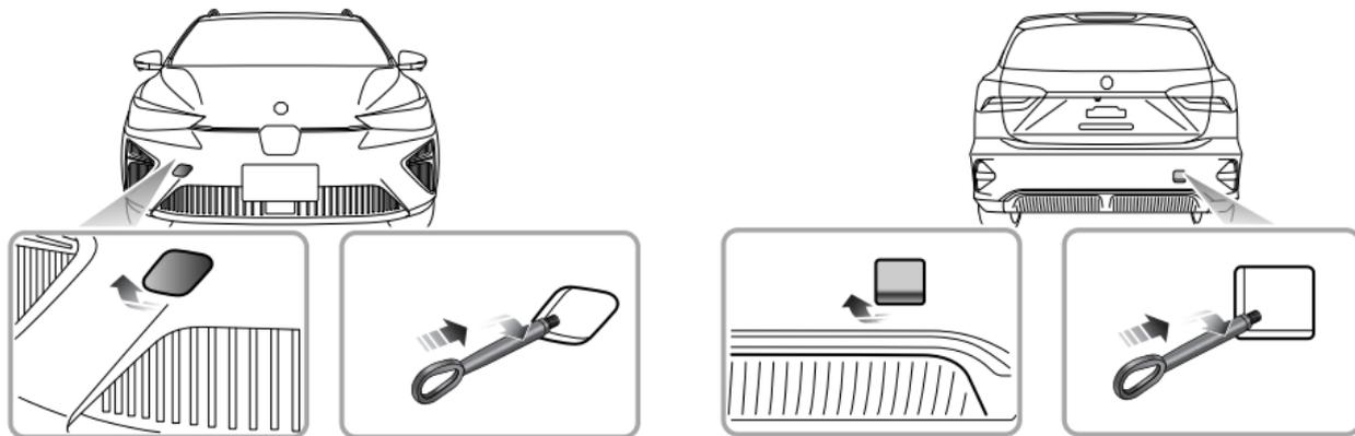
Your car is equipped with 2 towing eyes (located at the front and the rear of the vehicle), which are used for fitting the towing hook in the tool kit. The tool kit is placed beneath the loadspace floor.
