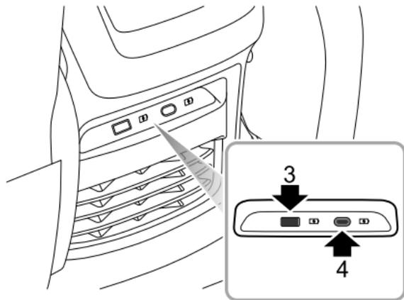
**Note:** Use of the USB port when the vehicle is not in READY mode will consume the battery power, extended use will cause premature discharging of the vehicle battery, and the vehicle may be prevented from being switched into READY mode.
