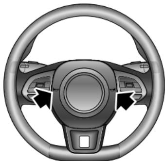
Press the horn button area (indicated by the arrow) on the steering wheel to operate the horn.
