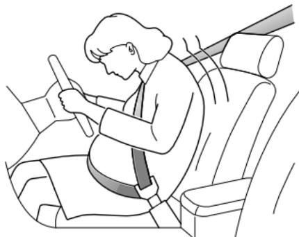
The diagonal section of the seat belt should pass across the chest as normal, the lap section of the belt should pass below the belly, low and snug on the hip bones. NEVER position the belt on or above the belly.
