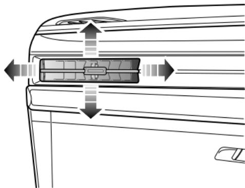
Slide the button in the centre of the louvres to the left or right to open or close the vent. Toggle it up and down, left and right to adjust the air direction.
