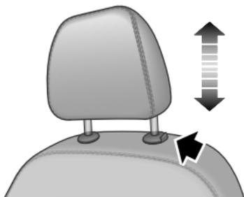
When adjusting a head restraint from low to high position, pull the head restraint directly upward, and gently press it downward after it reaches the desired position to make sure that it is locked in position. To remove the head restraint, press and hold the guide sleeve button (as indicated by the arrow) on the left of the head restraint, then pull the head restraint upward to remove it.
