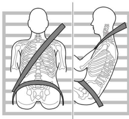
When wearing seat belts, the lap belt section should be positioned as low as possible across your hips. NEVER cross the abdomen. In the event of a collision, the lap belt can apply a force on the hips and reduce the possibility of
