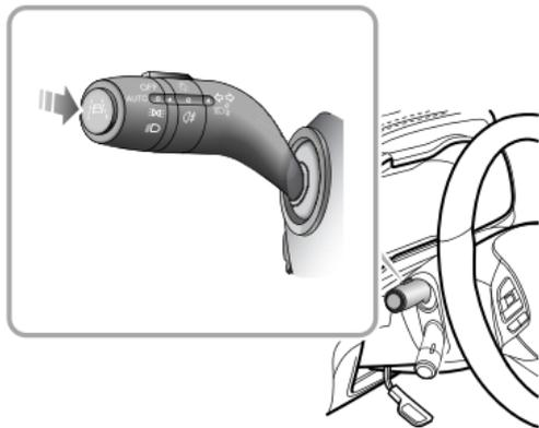
Having turned the lane assist system ON in the infotainment display, press the button at the end of the indicator stalk switch (as shown above), the system will enter the standby or active state.
