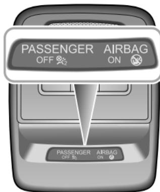
When the switch is turned to the OFF position, the OFF indicator light ( located in the PAB display panel in the lamp assembly ) illuminates, this indicates that the passenger airbag is disabled.
