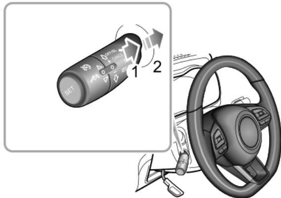
The traffic jam assist system switch is located in the infotainment display. Enter the corresponding interface for driving assistance to turn the system ON/OFF. Operating the adaptive cruise control level to “RESUME” twice will switch the traffic jam assist system to standby or active state.
