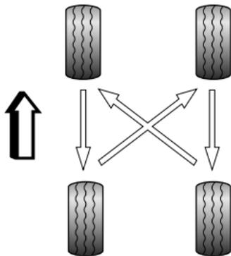
**Note:** Directional tyres (identified from the arrow on the tyre side) **CANNOT** be swapped from side to side.
