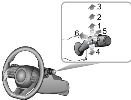
The front wipers and washers will only operate when the START/STOP Switch is in the ON/READY position. Operate the stalk switch to select different wiping modes:
